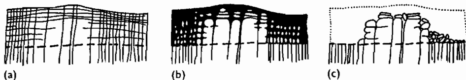
Fig-4 : Stages in the evolution of a group of tors, illustrating the importance of joint spacing
